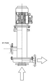
The length and diameter of the discharge pipe will determine the operating point of the pump. The pump selection is based on the information given together with the inquiry. It is therefore important that the discharge pipe work installation is carried out according to the same plans as those used for the pump selection. It is recommended to install a pressure gauge directly on the outlet of the pump.
