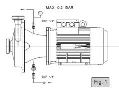
(Fig. 1) I.e., the throttle (not for the 60 series), supplied with the pump, is fitted to the bottom connection and connected to the water supply. The flow is set so that a small amount of water drips from the upper side ( $\pm$  10 l/hour). It is preferable to fit a hose at the upper connection so that any leakage can be sent to drain. Never put a valve or restriction in the drain side of the quench liquid or pressure may build up in the quench chamber.
