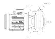
Make sure not to confuse the gas outlet and water inlet with the connection of the (optional) flushing double sealing.
