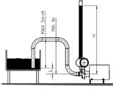
ing vessel, special attention has to be paid to the pipe work in case the pump is not installed with a flooded suction. The pipe work has to make sure there remains enough water in the pump casing when the pump is switched off to give the pump its air-handling capacity on the next start-up.
